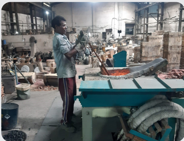
Figure 1: Charging into the furnace
